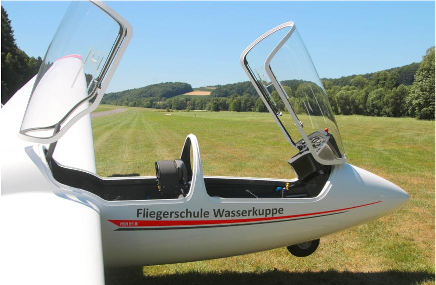
**Both canopies MUST BE CLOSED at all times**, except when getting in and out. Even walking a few feet away to hook up the ground or aero tow rope will leave the canopies exposed to damage.
